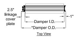
\*Recommended damper o.d. = Duct size -1/2"
