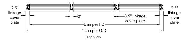
In Duct damper sizing for 3 or more sections wide TB-155,156 or SW-155, 156:
