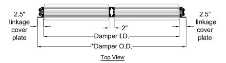
In Duct damper sizing for 2 sections wide TB-155,156 or SW-155, 156:
